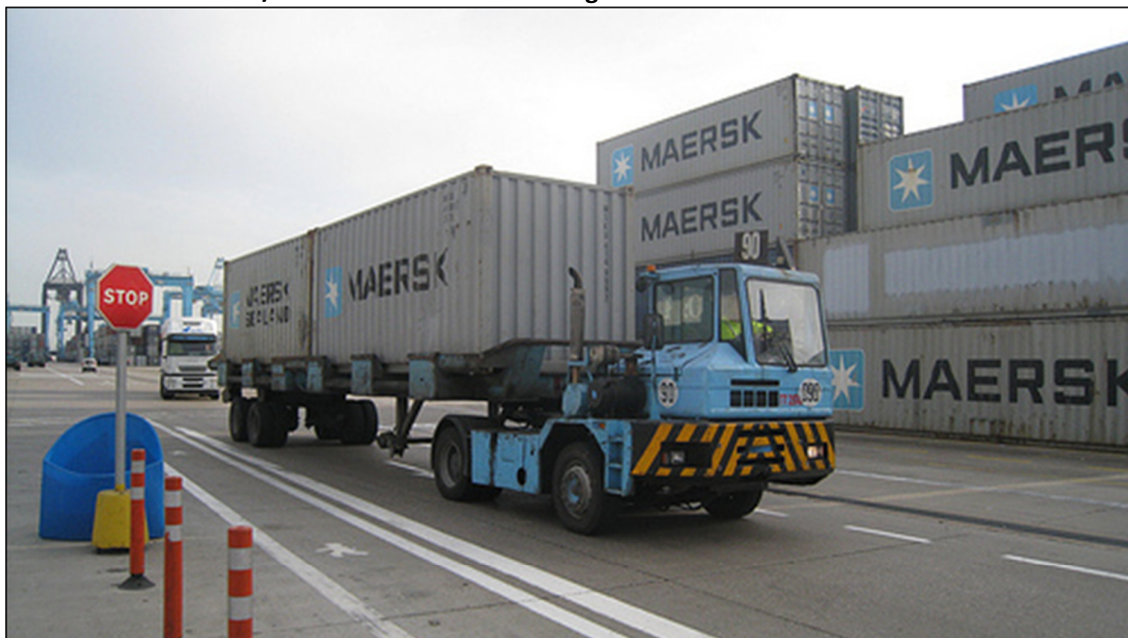
Picture 5: Yard Tractor/Skeletal Semi-trailer Moving Containers on Private Haul Road
