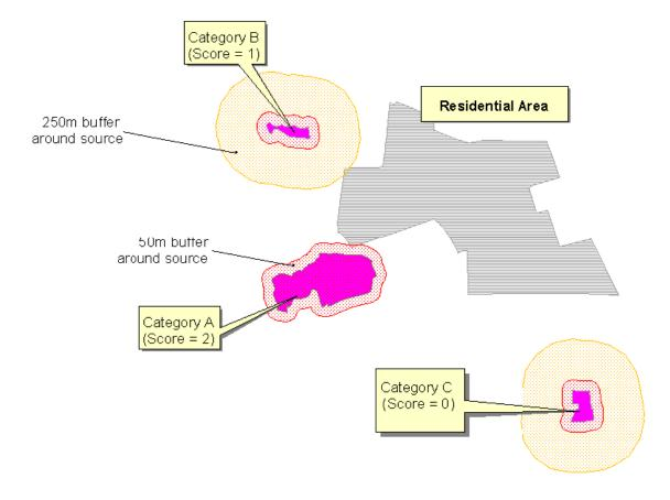
Figure 4.1 - Schematic diagram of proximity scoring method.
