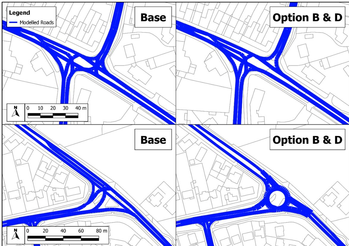
**Figure 4: Changes to road links in the Option scenarios; Right-hand turns removed from Marsh Drive at the A6/Church Road/Marsh Drive junction (top) and creation of a roundabout at the A6/New Road junction (bottom)**
