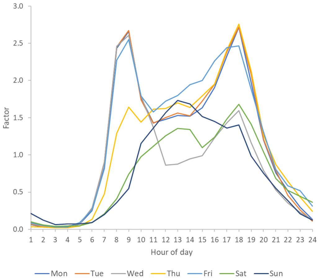
Figure 6: Diurnal profile for each day of the week used in the model, where the factor is the value that the average daily emissions are multiplied by in the model
