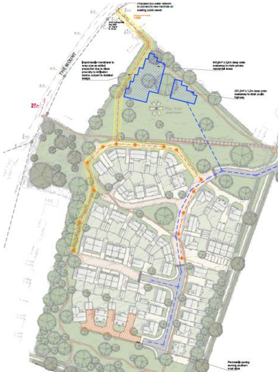
Figure 11: Extract from drawing number P16-120 200 rev B (Rodgers Leask) showing proposed drainage strategy contained within the revised FRA appendix K. Surface water drainage coloured blue (including two large soakaways to the north); foul drainage coloured orange
