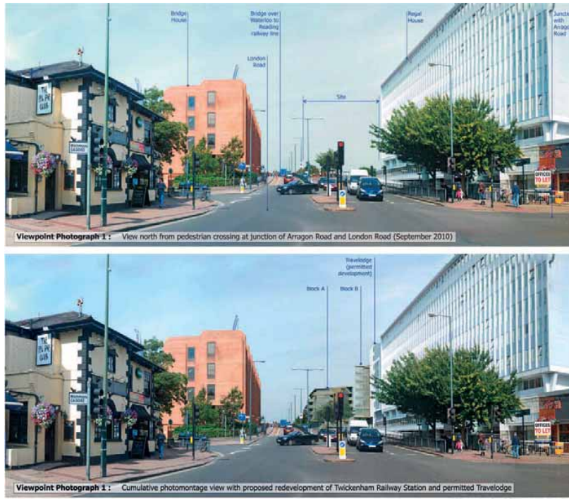
Figure 8.3 Cumulative photomontage of redevelopment at Twickenham Railway Station with other permitted development, a neighbouring hotel extension. Note the aspect ratio of the image to encompass the vertical field of view of the urban context; camera used in portrait orientation
