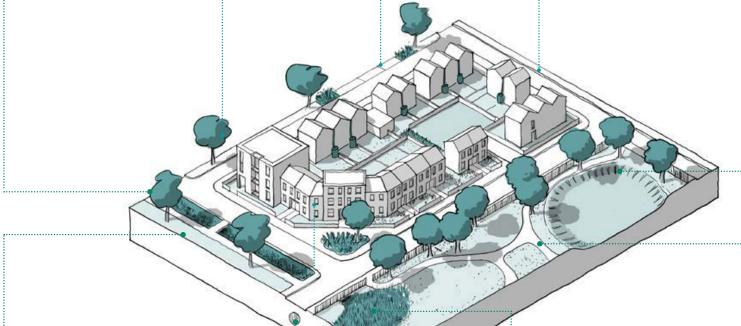
Swales: Shallow channels that provide attenuation while also channeling water to other features such as ponds.
