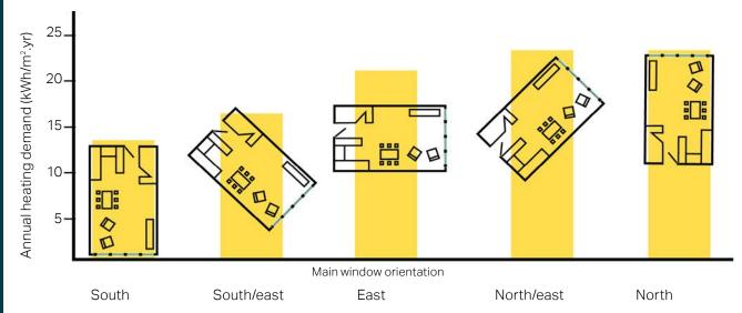
**Figure 34:** Illustrative graph showing solar orientation of a room against the annual heating demand.
